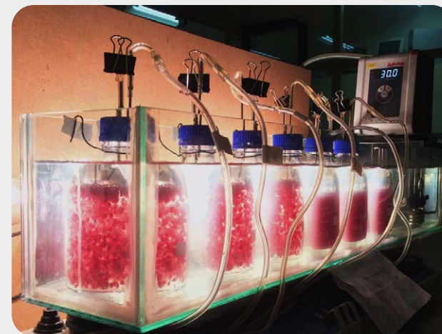
Top: Photofermentation using immobilised Rhodospseudomonas palustris Bench-scale.
