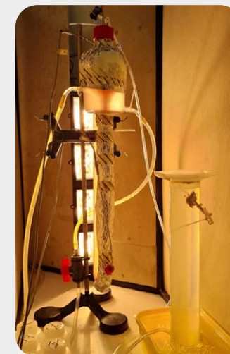
Top: Photofermentation using immobilised Rhodospseudomonas palustris Bench-scale.
