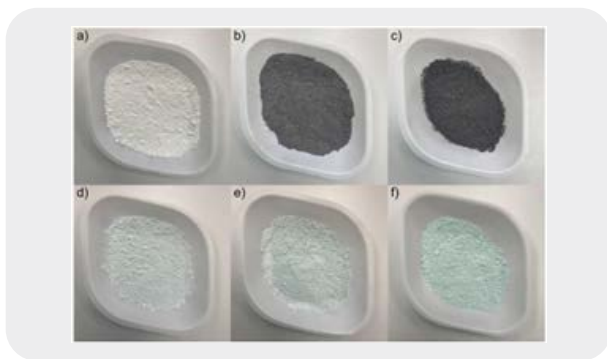
▲ \text{TiO}_2 nanoparticles with varying metal additives (from: Master thesis by Mr Van Den Berg, 2024, Cu and Pt loaded \text{TiO}_2 for \text{H}_2 production via photocatalytic ethanol reforming)
