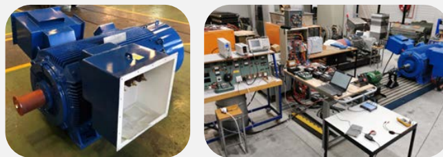
Synchronous condenser (the DC-VRM) being tested in the SU Wind-Energy-Spoke laboratory. ^
