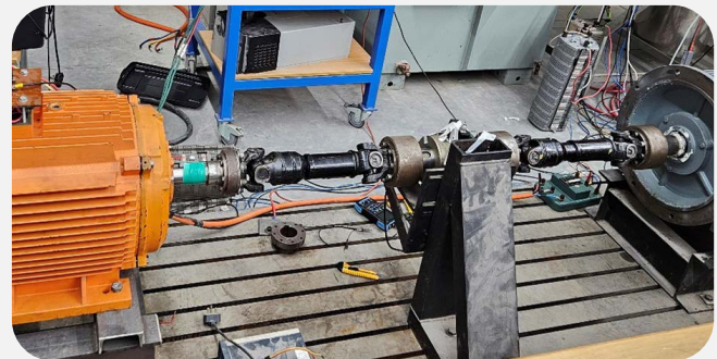
Test set-up for both BDFIG and BDFRG. ^
