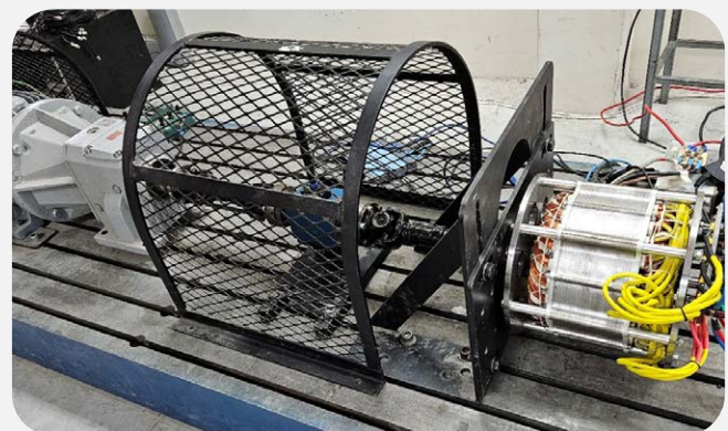
Test setup of the PMVG (right). ^
