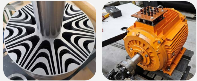
BDFRG rotor in manufacturing (left) and test machine (right). ^
