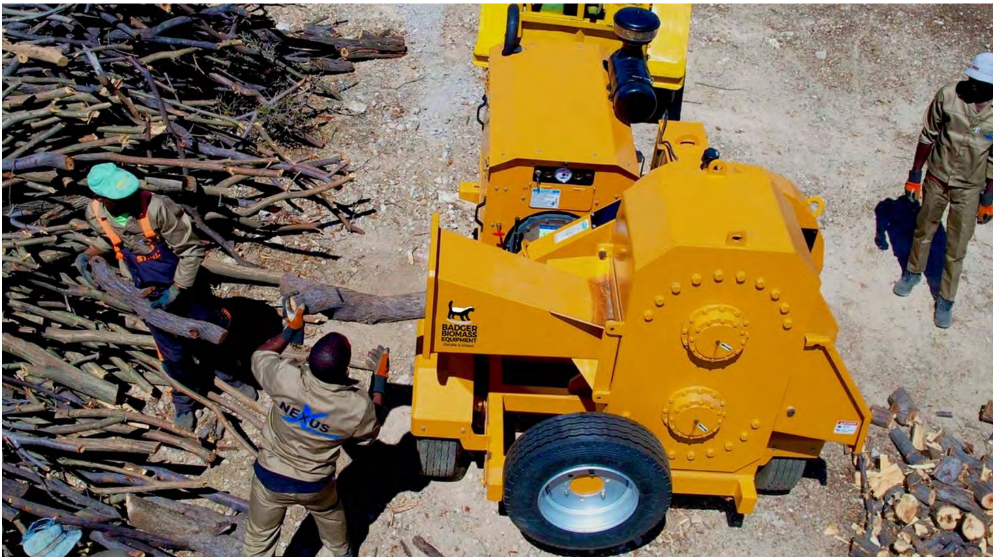
Photograph 1: Handfed Billeting Machine (Source: Africa Biomass Company, Worcester)
