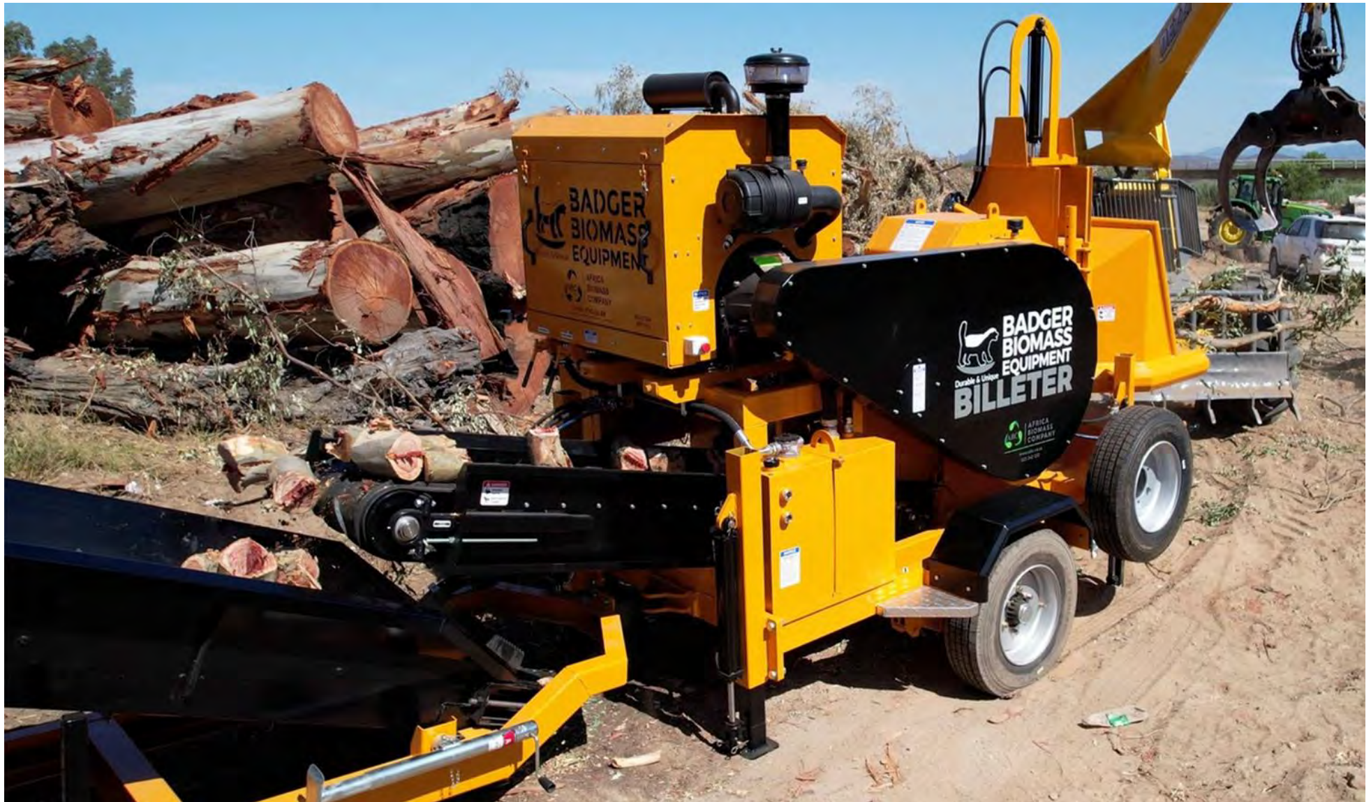
Photograph 2: Machine fed heavy duty Billeter capable of tree trunks and logs up to 200 mm diameter. See typical billets on discharge conveyor (left) [Source: ABC]
