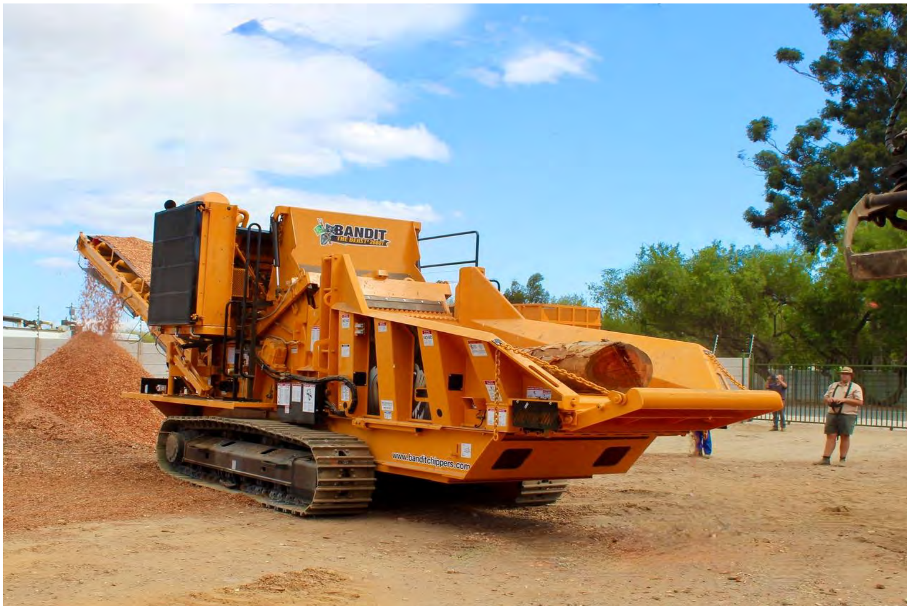
Photograph 1: Diesel driven BANDIT BEAST CHIPPER with horizontal grinder (Source: Africa Biomass Company [ABC], Worcester)
