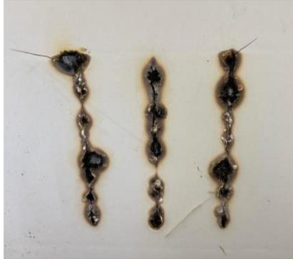
**Figure 1 Burnt back sheet of crystalline Silicon PV module.**
