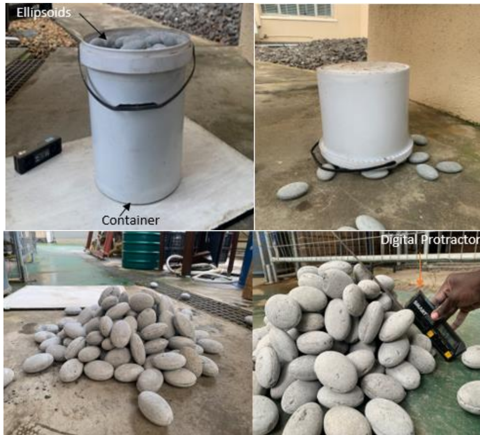
Figure 3. Illustration of determination of angle of repose
