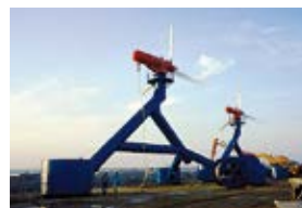
OUC 100kW tidal current device assembled
