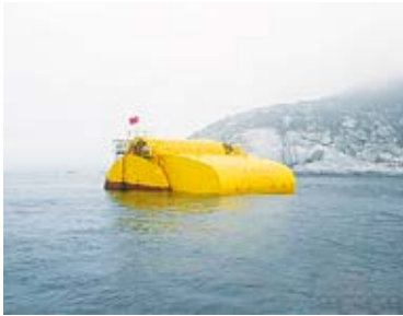
DUCK III 100kW WEC in test
