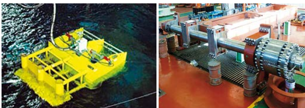
Pendulum Wave Energy Converter System and Rotary Vane Pump
