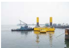
Haineng II 200kW tidal current device in the dock
