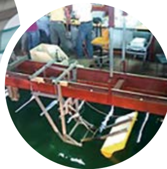
Wave tank test on 1:5 model scale
