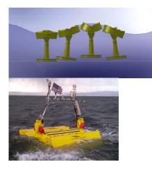
SeaRay is a two linkage attenuator. The PTO is linear permanent magnet.
