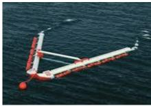
Weptos is composed of a V structure that faces into the oncoming waves. On the side of the V structure, Salter ducks span the length and are the primary wave energy converters. The inside of the ducks work on a ratchet mechanism that transfers the wave energy to a common axle.
