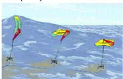
LOPF is like a "see saw" with a heavy generator on one end and the anchor on the other. All sized buoys can operate in all sea conditions beside that with floating ice. Buoys can ne unhooked form mooring for easy maintenance. At present there is 3 different sizes of buoy available ranging from 70 W to 5 kW. Survivability claimed for 15-20 years lifetime of buoy. Concept taken over by Resen Waves. <u>www.ResenWaves.com</u> and email <u>info@ResenWaves.com</u> [Sept 2013]
