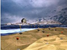
The Pelagic Power WEC consists of a linear piston pump, a water anchor and a surface buoy.
