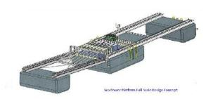
The **Sea Power Platform** Wave Conversion Device consists of a floating central inertial body about which are fitted power-producing floating bodies connected to the central body via the power take-off and damping system. The device consists of 2 pontoons- the Main pontoon and the Forward pontoon. The pontoon floats are manufactured in concrete and are thus very low cost.
