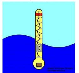
The module of FWEPS is an oblong axisymmetrical capsule-float which is located on the sea surface. Inside the capsule there is a mechanical wave energy converter, consisting of an oscillatory system and drive, and a linear generator and energy accumulator.
