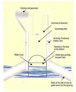
It is a floating device tethered with chains to piles driven to ocean bottom. The wave action raises the heavy partially buoyant piston that drives the overhead crankshaft by half turn. The receding wave drops the piston completing the balance half turn. One revolution is obtained for every wave. Using gear box and generator the current is produced continuously.
