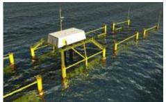
Langlee wave energy technology focuses on converting the horizontal sub-surface energy contained in ocean waves. The Langlee device orientates itself during wave loading. It uses a hydraulic P.T.O. A unit is typically 140m long and 25m wide.
