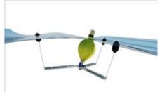
Once on site, an inflatable absorber that looks like a large balloon is filled with water. Sitting just under the surface, the absorber is moved by passing waves – and the energy from this motion drives a generator to produce electricity.
