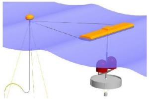
The focus of the device is on the dominant wave direction and wave crest length by use of a wider float, the use of a double acting pump, a buoyancy controlled water anchor and a PTO consisting of accumulator, water turbine and generator. Using a wider stabilized float, results in a wider wavefront being captured and hence more energy being harvested. The PTO has hydro-power similarities, and is disconnected from the moorings.
