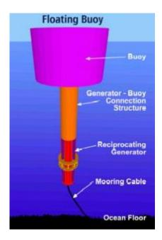
Electric Buoy - The Generator housing moves up and down with the motion of the Buoy on the ocean's surface while the Damping Plates hold the Generator Coil in a stable position. The relative motion between the magnetic field in the generator housing and Generator Coil creates an electric voltage in the Generator Coil.
