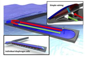
Bombora is similar in design as the SWEC with the distinct difference of having a flexible membrane that pumps and sucks air locked in the caisson chambers.
