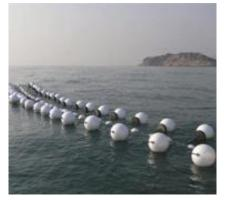
The Motorwave consists out of 70 PVC buoys. Each buoy has a volume of  $4 \text{ m}^3$ . A MotorWave unit can pump water 50 m high by using wave action to crank a uni-directional gear, like a bike pedal.
