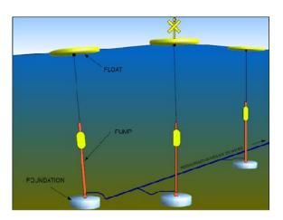
A float travels up and down with the waves and operates a pump to pressurise sea water which is piped ashore. Many individual pumps are connected together to produce substantial amounts of pressurised water.
