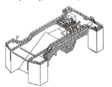
FWPV is an overtopping device for offshore operation developed by Sea Power International, Sweden. It consists of a floating basin supported by ballast tanks in four sections. A patented anchor system allows the orientation of the vessel to the most energetic wave direction. A pilot plant has been developed and deployed in the '80s near Stockholm, Sweden while a 1.5 MW vessel is planned to be deployed at 50-80 m depth 500 m offshore Mu Mess, Shetland.
