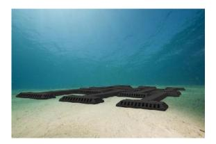
Unlike floating buoys or Aquamarine Power's signature "Oyster" design, both proposed in Oregon, M3'S design doesn't pierce the surface of the ocean or impact coastal views. Instead, it sits on the ocean floor at depths between 50 and 100 feet. It generates power by responding to water pressure from the waves above, which alternately inflate and deflate a pair of airbags that turn a central turbine to generate power.
