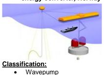
The system consists of a float, double acting pump, buoyancy controlled water anchor and PTO consisting in accumulator, water turbine and generator. 1:30 scale tests conducted in their home made wave tank. WAMIT model of float developed by Marintek in Sintef.
