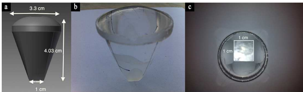
Figure 9: (a) Schematic diagram and (b), (c) photograph of the refractive secondary.
