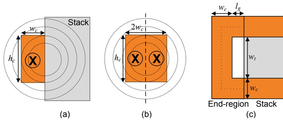
**Figure 5: (a) Conductor placed next to permeable lamination stack, (b) two conductors placed next to each other in air to form one large conductor and (c) dimensions for the end-winding inductance calculations.**
