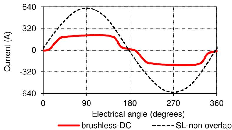
**Figure 12: Current versus slip for the non overlap SL and brushless-DC slip-PMGs.**
