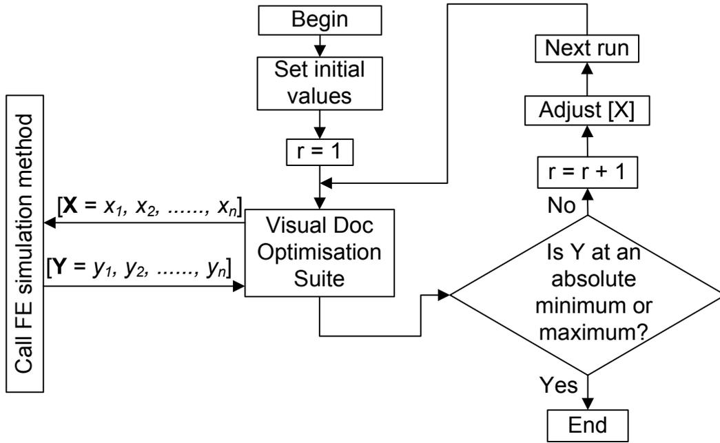
**Figure 7: Basic overview of machine design optimisation.**
