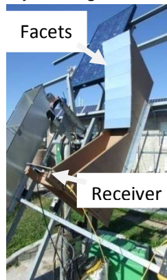
Figure 2: Module 1 installed on a dual axis tracker showing one side of the parabolic concentrator element.
