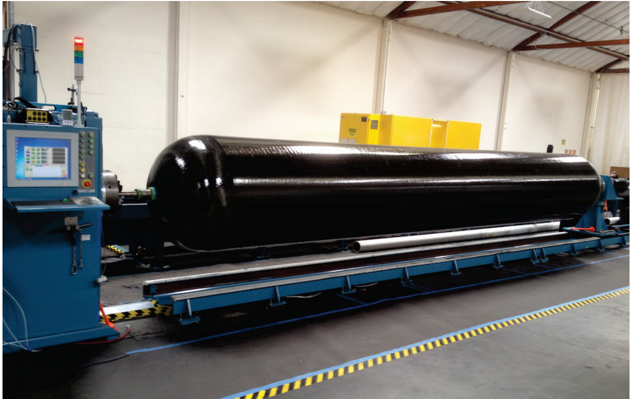
25-ft composite carbon fiber tank for high-pressure air storage.
