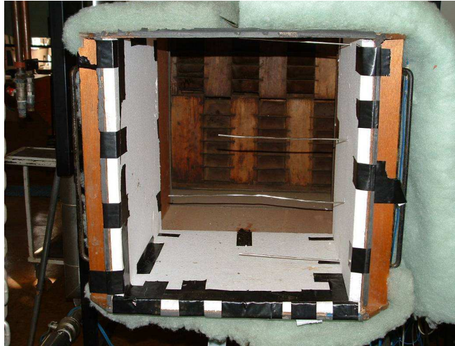
Figure 51: Wind tunnel wall insulation with mixer visible
