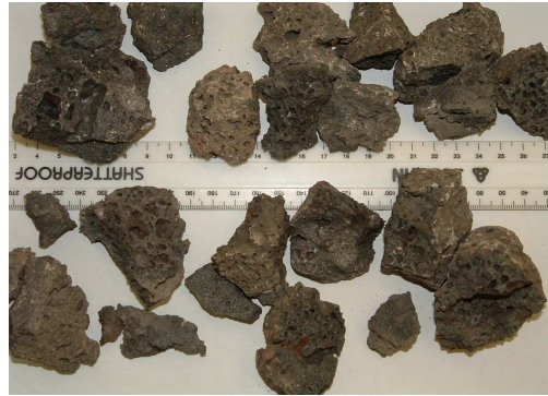
Figure 33: Fragmented slag sample after 60 cycles
