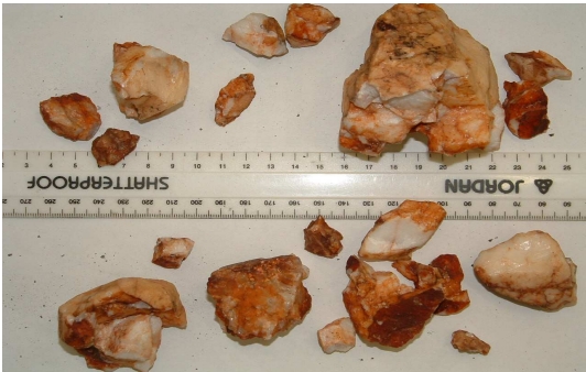
Figure 34: Fragmented quartz sample after 30 cycles
