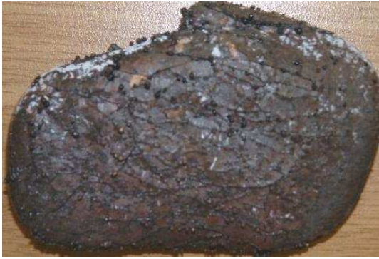
Figure 32: Structural failure of shale above 500 °C
