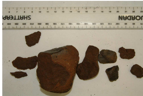
Figure 35: Dolerite explosive failure during first heating
