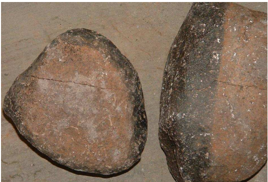
Figure 36: Hairline fracture of dolerite after 110 cycles
