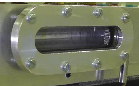
Figure E.2 Photographs of refrigerant injection, boiling and pulsing with excess mass. Flow is from left to right. Video of this process is given on the disk in Appendix G.
