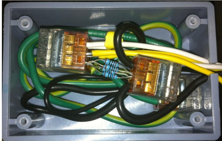
Figure E.3 Pull down resister of 10\text{ k}\Omega grounds floating signals present in PWM.
