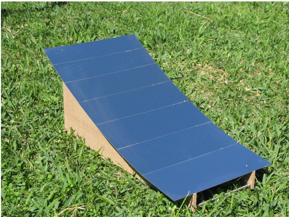
Figure 3.4: Constructed 7-facet reflector system
