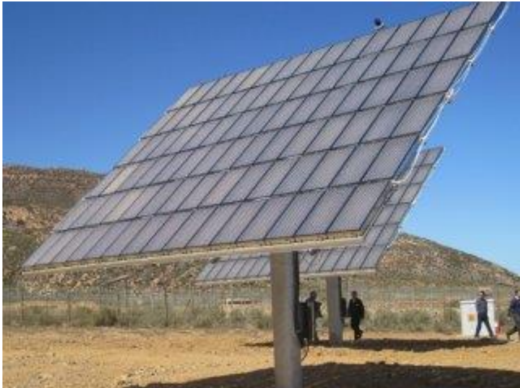
Figure 2.1: HCPV system mounted on a 2-axis tracker system at Aquila Game Reserve in South Africa [4]
