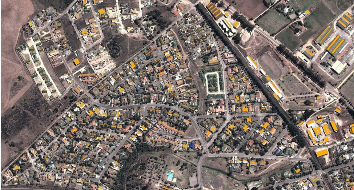
Figure 1: GIS Study results of Hessequa PV study (The yellow roofs were identified in Riversdale as suitable for the installation of a rooftop photovoltaic system.)
