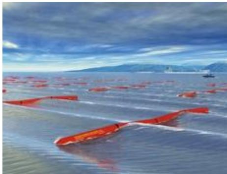
It is a semi submerged system that consists of several cylindrical sections (made out of steel) that are connected with hinged joints. Hydraulic pumps are used to utilize the bending motion inside the joints, which is caused by the passing waves. The high pressure oil is used to generate electricity in a hydraulic system.
