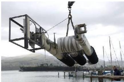
WET-NZ is a subsurface device that is designed to convert kinetic and potential wave energy. One module has a 500 kW generation capacity. It uses a direct-drive P.T.O and will be deployed in water depths ranging from 20 – 100m.
