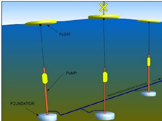
A float travels up and down with the waves and operates a pump to pressurise sea water which is piped ashore. Many individual pumps are connected together to produce substantial amounts of pressurised water.
