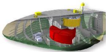
The Penguin is a floating device, weighing 1600 tons, 30 m long with three point mooring. Extends 2 m above water surface. Utilises wave's orbital velocity to spin flywheel connected to electric generator. Sea trials 20 June 2011 at EMEC.
