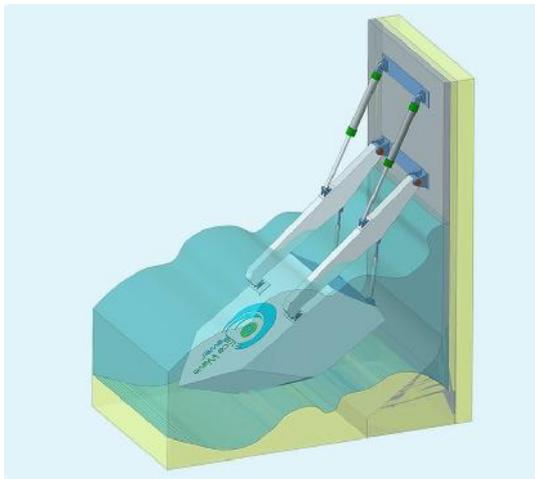
The EWP convertors draw energy from wave power throughout uniquely shaped buoys, “The Wave Clapper” and the “Power Wing” that rise and fall with the up and down motion, lifting force, change of water level, hydraulic air lock, and incident flux of waves.
