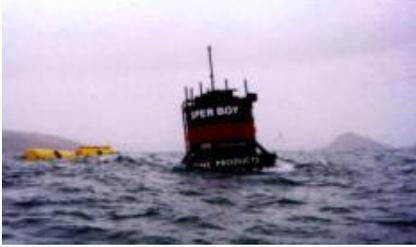
The Sperboy operates on the 'oscillating water column' principal. It uses buoyant material to keep it a float and several cables to keep it at a constant height. There is an air column on the inside of the device that oscillates as the waves passes. The energy is extracted from the oscillating air by turbines that in turn transfer the energy to generators.
