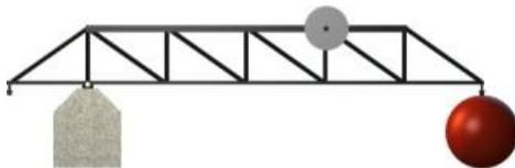
A float, at the end of a truss, is used to cause a “teeter-trotter” effect in the truss. The truss is allowed to pivot at the hinge point that’s situated at the base (the base is situated on the beach).
