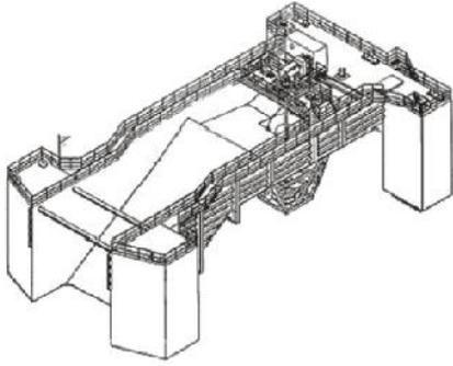
FWPV is an overtopping device for offshore operation developed by Sea Power International, Sweden. It consists of a floating basin supported by ballast tanks in four sections. A patented anchor system allows the orientation of the vessel to the most energetic wave direction. A pilot plant has been developed and deployed in the '80s near Stockholm, Sweden while a 1.5 MW vessel is planned to be deployed at 50-80 m depth 500 m offshore Mu Mess, Shetland.
