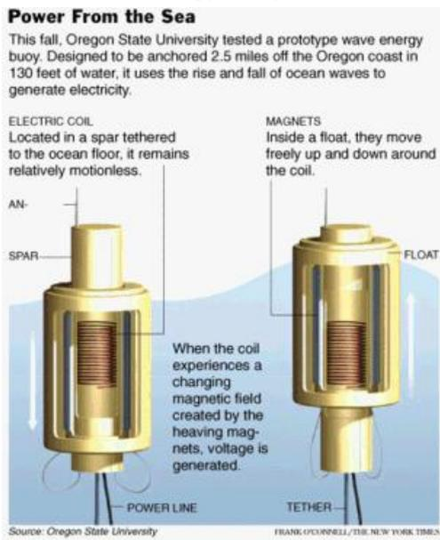
The buoy has permanent linear magnets that are attached to the shaft. These magnets induce a current in the coil that's housed inside the buoy. This unregulated AC voltage (from the buoys) is fed via a cable to a junction box on the seabed where it is converted to 12000V DC. The DC voltage will be changed back into AC on the shore before it's fed into the grid.
