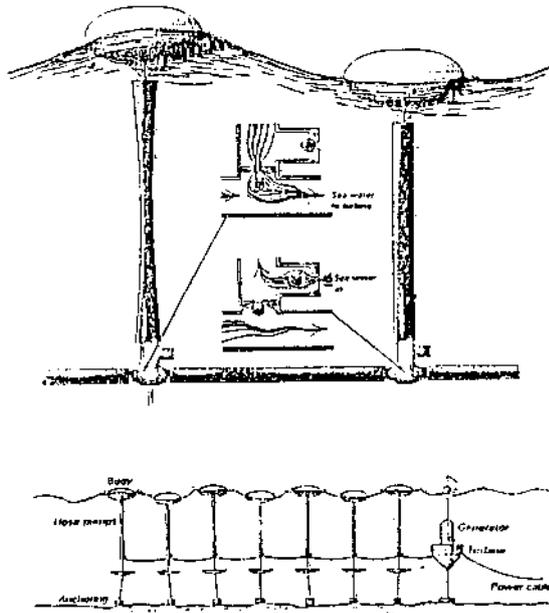
The Swedes use a hose pump, which is inserted between the float and a large damper disk, which is slack anchored to the seabed. When the waves lift the float, the hose is lengthened, and its volume is reduced. Hereby the water is pressed out and accumulated in a hose, that transport water from several pumps to a joint high pressure water turbine. When the wave lowers the float, the hose turns back to its original volume, and sea water is drawn in through valves.
