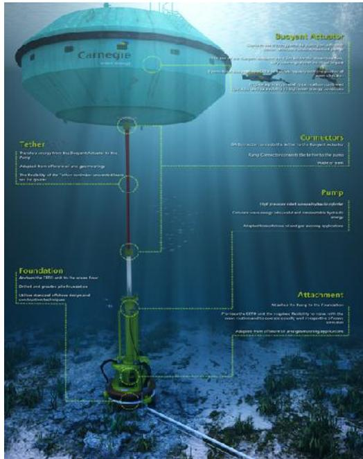
Fully submerged buoy (1-2 m below the surface) tethered to a seabed mounted pump. The unit delivers high pressure fluid ashore via a subsea pipeline, the high pressure fluid drives hydroelectric turbines onshore generating electricity or direct desalination of water. The buoy captures the wave energy thus pulling on the flexible tether driving the seabed mounted pumps.
