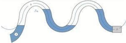
The WEC is a flexible hose that is designed to span several wave periods. The hose has a water and air intake at one end and is connected to a 'power module' at the other end. The higher pressure wave crests progress from the hose inlet to its' outlet moving the trapped water and air in front of the crest towards the outlet similar to a screw effect..
