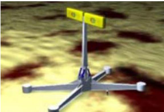
The EB Front is a small seabed-mounted bottom-hinged WEC. Similar to the WaveRoller, Oyster and Bio-Wave. Converts energy contained in surge as apposed to heave.
