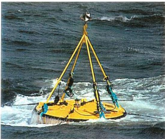
The wave power converter consist of a float 2.5 meter in diameter, connected by a rope to a seabed mounted piston pump, installed on 25 meter deep water 2,5 km from shore. The converter is designed to absorb an average maximum power of 1 kW.
