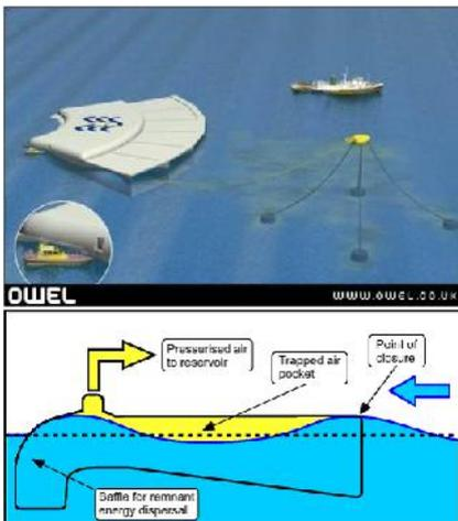
The WEC is a horizontally floating duct which is made up of several sections which together forms one large system. The height of the duct, at the entrance, will be equal to the average wave amplitude and the length will be determined by the average wave length. The fact that the system consists of several sections and that it is longer than the average wave length, will allow it to be stable. The anchoring system allows the WEC to align itself with the incoming waves.
