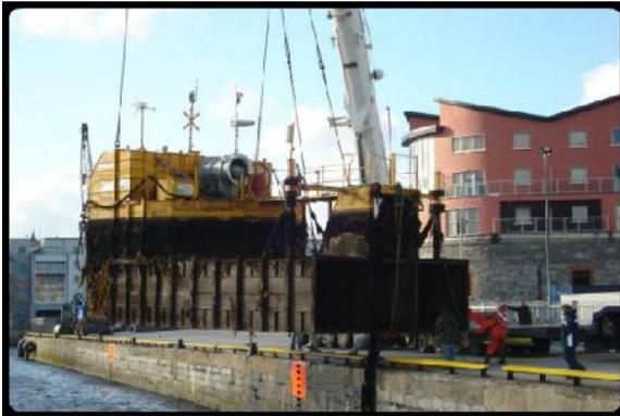
Floating OWC. Has an 'L' formation, where the water enters into device from the long side of the L. Survivability has been tested in arctic oceans and has been proven.
