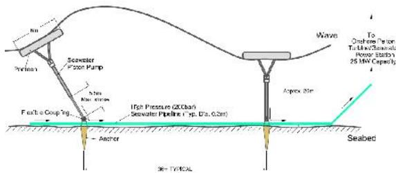
SurfPower is a pontoon anchored to the seabed via hydraulic cylinders that operates as a piston pump. Upward and lateral motion of the pontoon forces fluid from the piston pump, at high pressure, (200 bar) to a collection main on the seabed. This high pressure fluid is delivered to an onshore pelton turbine that drives an asynchronous electrical generator.
