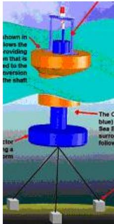
The Aegir Dynamos' two major components are the buoyant base (that is anchored by three cables) and the float that moves up and down with the swell. The linear motion between the float and the base is converted into angular momentum (the details of this conversion process is unknown to the author). The angular motion is then used to drive the generator that is sealed inside the central column.
