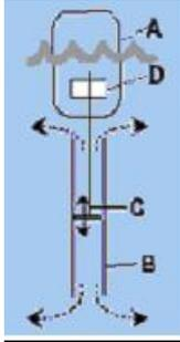
The buoy consists of three different parts: a buoy A, acceleration tube B and a piston C. The passing waves cause the acceleration tube to move relative to the water column inside it. The water (that is trapped inside the column) forces the piston to move relative to the acceleration tube. The up and down movement of the piston is converted to rotational energy by a mechanical system. This rotational energy is used to drive a turbine (no D).
