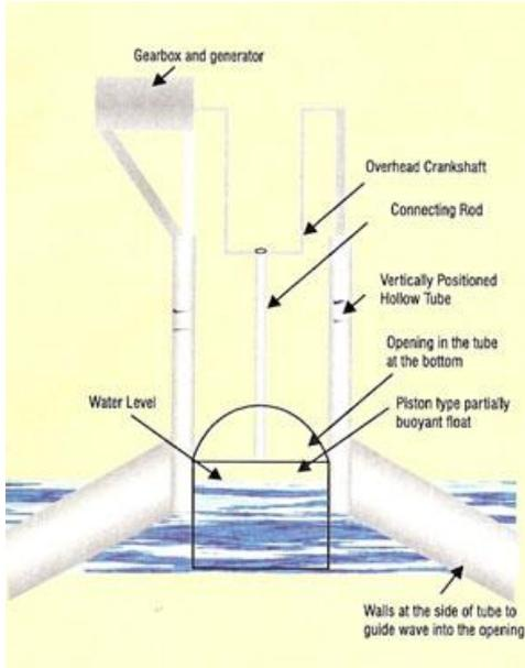
It is a floating device tethered with chains to piles driven to ocean bottom. The wave action raises the heavy partially buoyant piston that drives the overhead crankshaft by half turn. The receding wave drops the piston completing the balance half turn. One revolution is obtained for every wave. Using gear box and generator the current is produced continuously.
