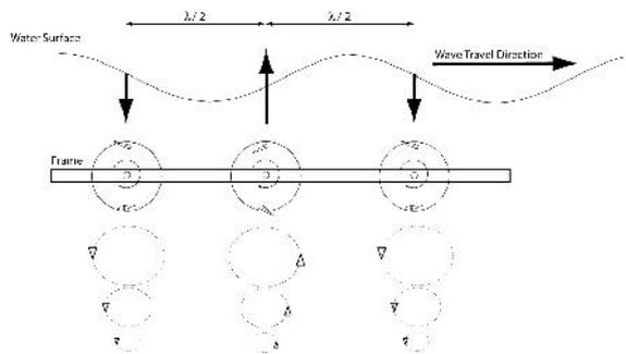
Two hydrofoils that rotate around a shaft aligned with the wave crests and operated under feedback control achieve wave termination
