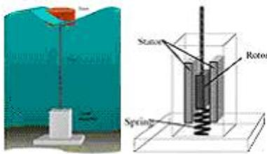
The system uses a three-phase permanent magnet linear generator to generate electricity. The linear generator is mounted on the seabed and it is driven by a floating buoy.
