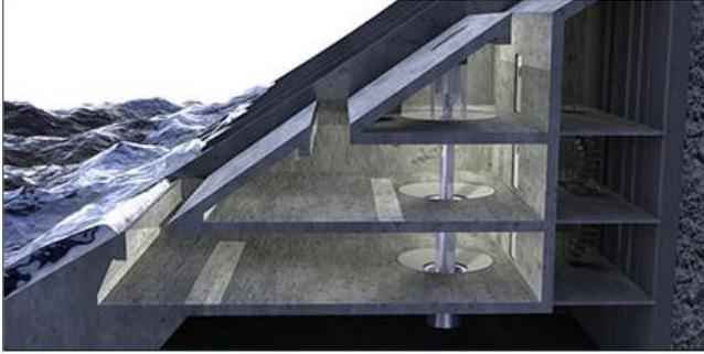
The SSG concept is based on the over topping principal. The system uses a total of three reservoirs placed on top of each other to capture the crest of the incoming wave and a specially designed multistage turbine to convert the head into mechanical energy (the system will operate very similar to a conventional hydropower station). The turbine will be connected to an electrical generating system in order to generate electricity for the grid, or to generate hydrogen.
