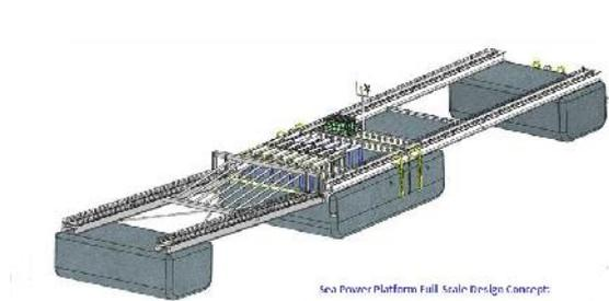
The **Sea Power Platform** Wave Conversion Device consists of a floating central inertial body about which are fitted power-producing floating bodies connected to the central body via the power take-off and damping system. The device consists of 2 pontoons- the Main pontoon and the Forward pontoon. The pontoon floats are manufactured in concrete and are thus very low cost.
