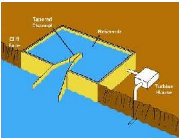
The system has a tapered channel that leads up to an elevated reservoir. The channel focuses the waves as it gets narrower, this effect allows the waves to flow into the elevated reservoir. The elevated water will be used to drive a conventional hydropower plant as it's allowed to flow back into the ocean.
