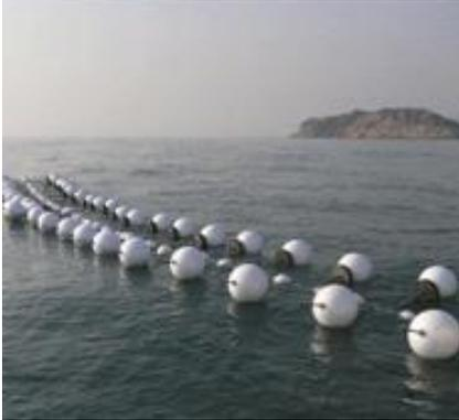
The Motorwave consists out of 70 PVC buoys. Each buoy has a volume of 4 m<sup>3</sup>. A MotorWave unit can pump water 50 m high by using wave action to crank a uni-directional gear, like a bike pedal.
