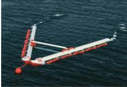
Weptos is composed of a V structure that faces into the oncoming waves. On the side of the V structure, Salter ducks span the length and are the primary wave energy converters. The inside of the ducks work on a ratchet mechanism that transfers the wave energy to a common axle.
