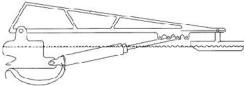
A set of connected articulated floats flex when the waves pass under them. This bending motion is used to drive piston pumps which pumps seawater under high pressure to the shore where it is used to drive a turbine. This turbine powers a generator.
