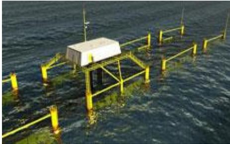
Langlee wave energy technology focuses on converting the horizontal sub-surface energy contained in ocean waves. The Langlee device orientates itself during wave loading. It uses a hydraulic P.T.O. A unit is typically 140m long and 25m wide.
