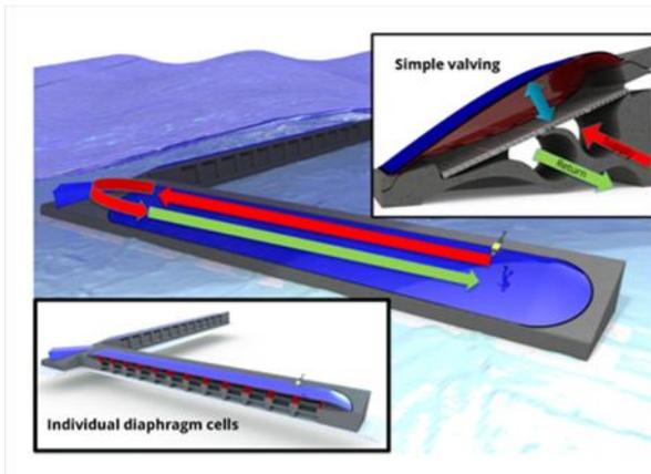
Bombora is similar in design as the SWEC with the distinct difference of having a flexible membrane that pumps and sucks air locked in the caisson chambers.
