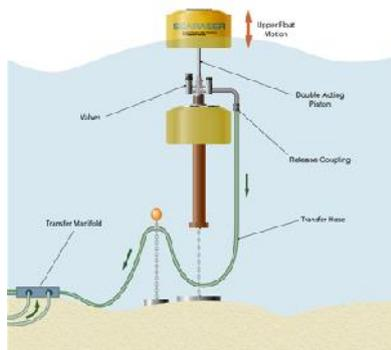
Searaser is buoy type device consisting of top float, double acting piston, reactor float and single point mooring. The device pumps high pressure seawater which can be stored in a reservoir (50m head has been achieved). During sea trials in April 2009 the prototype 83 delivered 0.77kW of power. Similar to CETO and Seadog.
