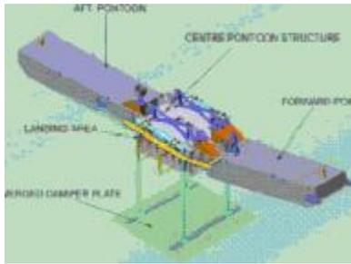
The device consists of three steel pontoons that point into the wave direction. There is a damping plate attached underneath the central pontoon in order to increase its inertia, therefore it will stay relatively still.
