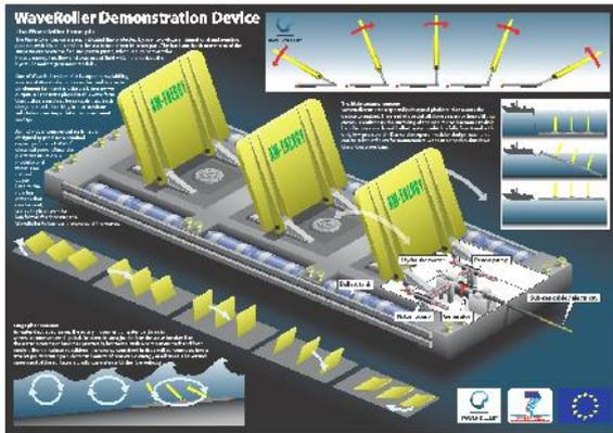
WaveRoller is a device that converts ocean waves to energy and electricity. The machine operates in near-shore areas (approximately 0.3-2 km from the shore) at depths of between 8 and 20 meters. It is fully submerged and anchored to the seabed. A single WaveRoller unit (one panel) is rated at between 500kW and 1000kW, with a capacity factor of 25-50% depending on wave conditions at the project site.
