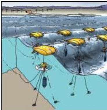
Couples to up/down motion of heave based systems. A shaft transfers wave motion to the MHD generator which is deep underwater (no wave motion). The shaft forces the conducting fluid through powerful permanent magnets. Low voltage/high current electrical energy is generated via the MHD interaction. An electrical inverter converts the electrical energy to commercial quality 60 Hz AC power. Power is transmitted to shore from multiple generating stations and connected to the grid.
