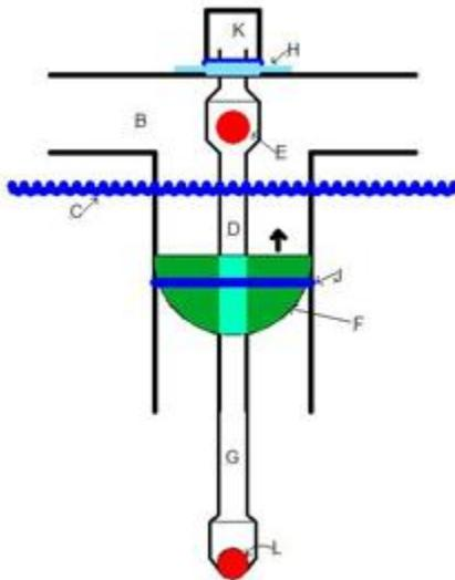
**The OWWE (Ocean Wave and Wind Energy)** The picture shows a hybrid wave and wind power rig called 2Wave1Wind. 10 modules of 600m can produce 1 TWh a year at the price of £ 0,04/kWh in wave climate of 40 kW/m wave front.
