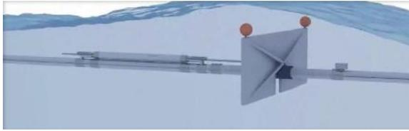
The system is built from prefabricated modules that can be produced at a low cost. Each module consists of an energy collector and a simple pump. The energy collector is a plate that can slide back and forth. The pump consists of a cylindrical chamber with a piston inside that is powered by the movement of the energy collector.
