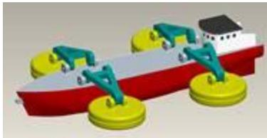
Mobile wave energy harvester proposed by Fraunhofer Center for Manufacturing Innovation. The vessel contains a PTO system (most likely hydraulic) and banks of batteries. Wave energy is captured by pontoons attached by lever arms to the ship. Vessel must travel from the low energy area of the port to an area of higher energy to feed generated power into grid. This mobility increases survivability, but also fuel costs. Sailing crew inactive during times of energy capture.
