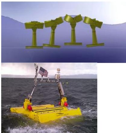
SeaRay is a two linkage attenuator. The PTO is linear permanent magnet.
