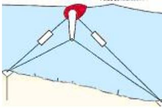
The passing waves cause the Duck to rotate in a nodding motion; this motion is used to pump hydraulic fluid or to compress air. If the hydraulic principle is utilized the fluid will drive a hydraulic motor which in turn drives an electrical generator in order to generate electricity, but if air is used the compressed air will drive a turbine.
