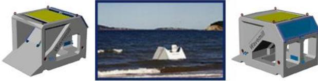
The Wavemill is designed for nearshore and shoreline applications. The device consists of a curved wall which focuses incoming waves to drive seawater through a hydraulic pump. According to the IEA the pressurised seawater can be used for desalination (20 L/s) or electricity generation (up to 233 kW). Wave tank testing was done in 1998 and a small desalination unit was deployed in Nova Scotia in 2001.
