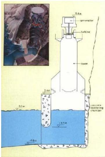
Kvaerner Brug's MOWC consists of a hollow concrete chamber with surmounted cylindrical steel tower approximately 10 m tall. The device has a half U-tube shape to promote resonance and uses a Well's turbine.
