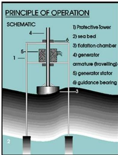
DECM is a neashore point absorber with a linear generator P.T.O. It consists out of a floatation unit that oscillates relative to a fixed reference. The floatation unit is hoisted above the sea level during extreme storms to ensure survivability.
