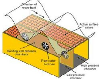
The pressure difference between the two chambers is utilized by several turbines. These turbines powers generators in order to generate electricity.
