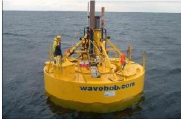
The WaveBob is a free floating point absorber that uses a hydraulic system to convert the energy of the waves into electricity (there is very little available information about the system). The hydraulic system uses biodegradable fluids in order to prevent pollution in case a leakage occurs.
