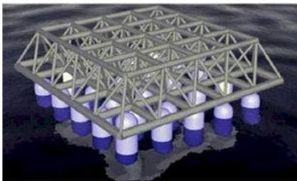
The system consists of a series of bobbers that's attached underneath a platform. The bobbers will harness the up and down motion of the waves in order to generate electricity (the exact principal is unknown to the author). The rig will be allowed to float freely, allowing it to harness waves from any direction.
