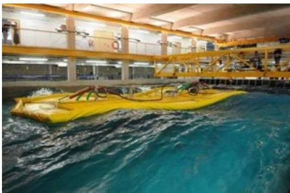
The device works like a typical linear generator in which a set of magnets mounted in a translator is moved up and down inside multiple coils of wire of an armature. However, there is a crucial difference with Snapper: alongside the armature coils is a second set of magnets of alternating polarity.
