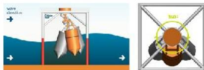
The WEGA device is an articulated suspended body, semi-submerged, attached to a mount structure, which oscillates in an elliptical orbit with the passage of waves. The PTO is located on mount structure above water reducing exposure to the corrosive environment and easing accessibility for maintenance.
