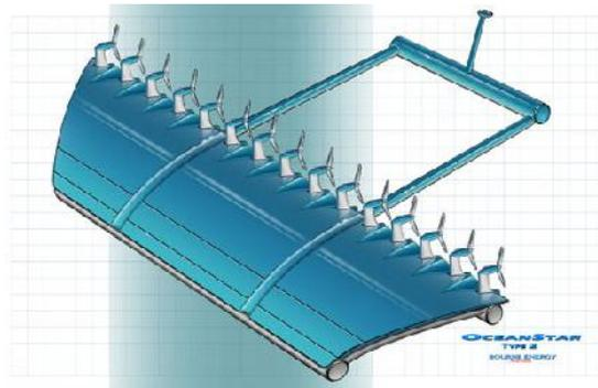
The Oceanstar is a submerged WEC that utilises sub-surface pressure to drive multiple turbines.
