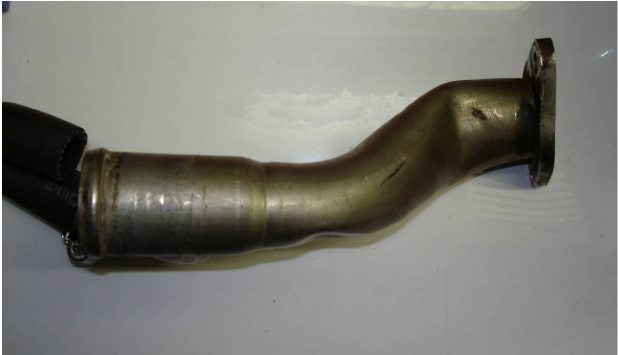
Figure 4-1: Damaged coolant outlet pipe limiting flow
