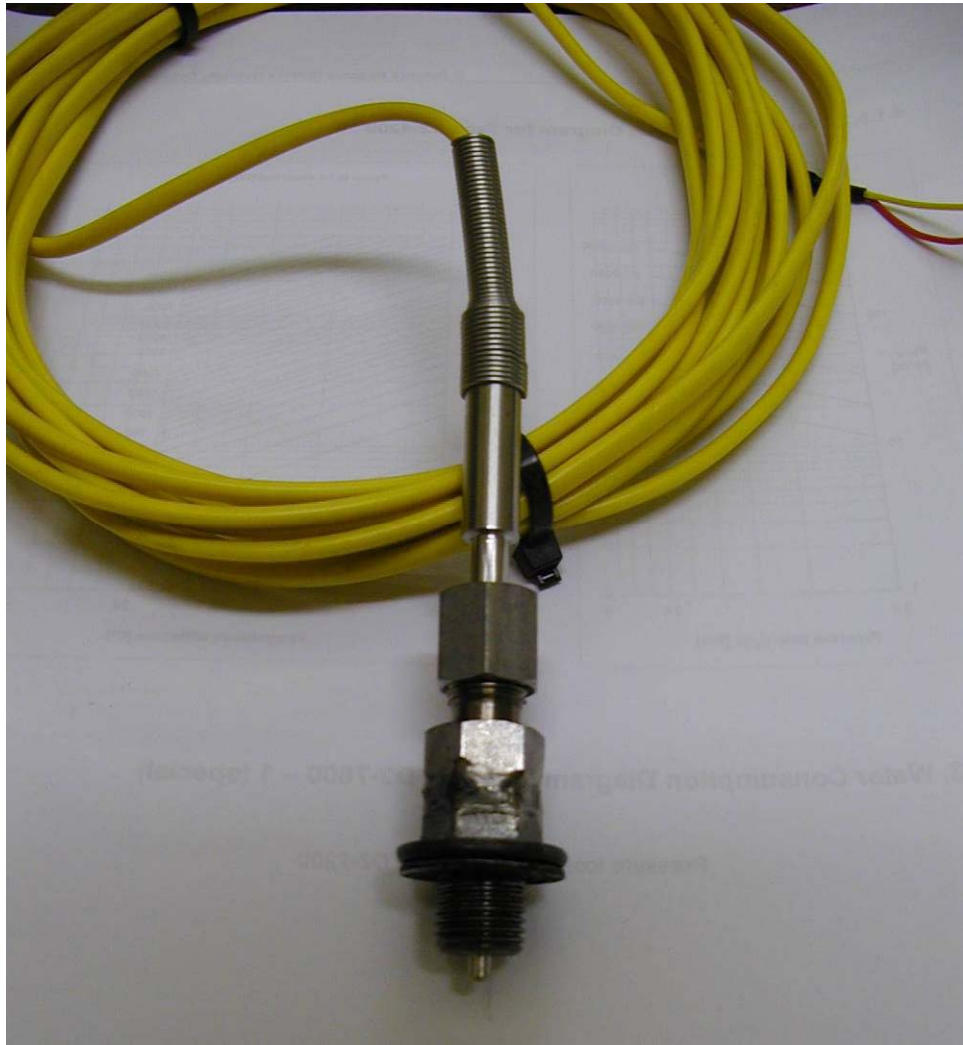
Figure 3-10: Sump plug with thermocouple
