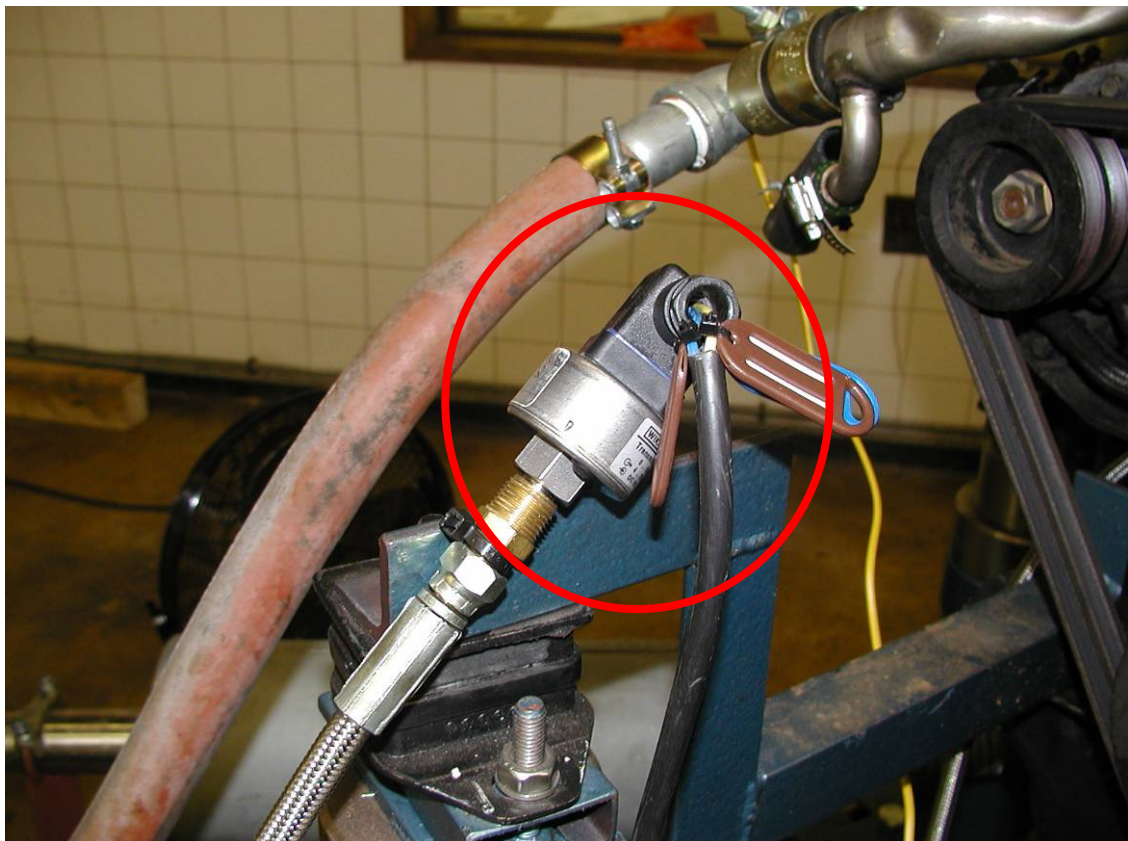
Figure 3-8: Oil pressure transducer connected to braided hose
