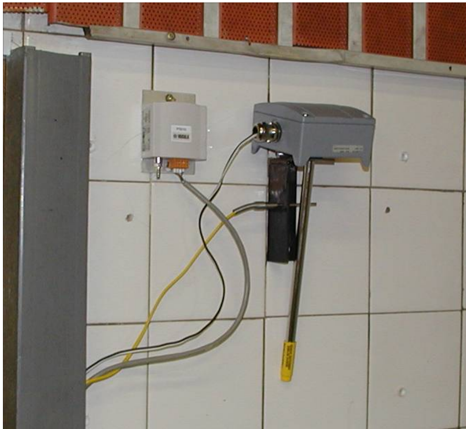
Figure 3-33: Ambient pressure sensors; barometric pressure on the left, humidity probe above right and the thermocouple
