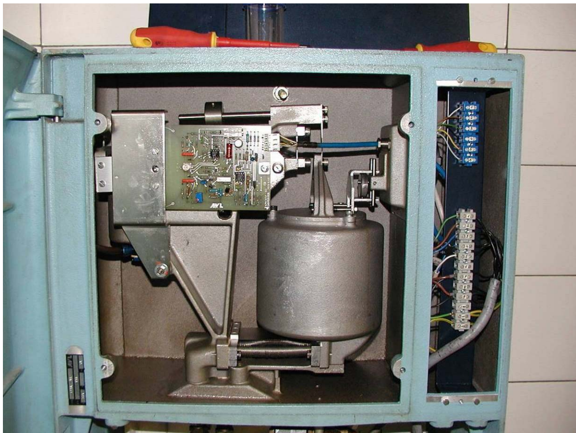
Figure 3-18: AVL internal view of the vessel and electronics
