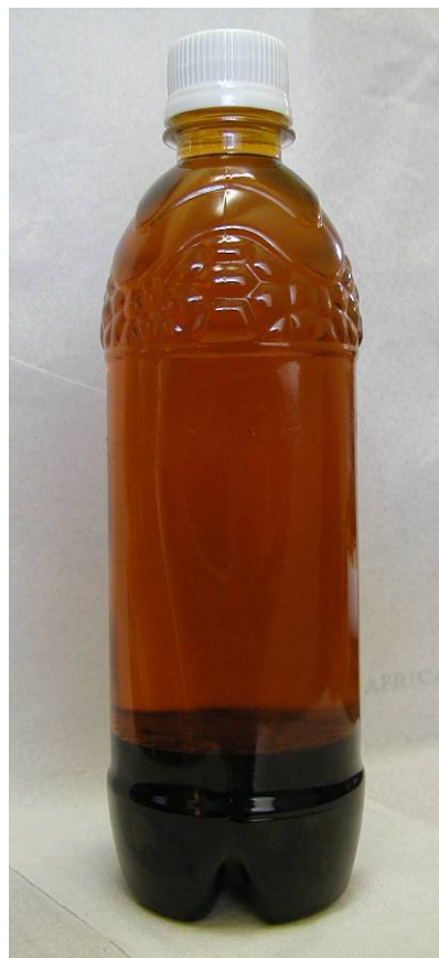
Figure 2-1: Sample showing biodiesel on top and glycerol at the bottom
