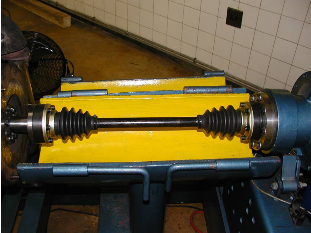
Figure 3-16: Cardan shaft coupling (Figure 3-17 shows the closed protective housing)
