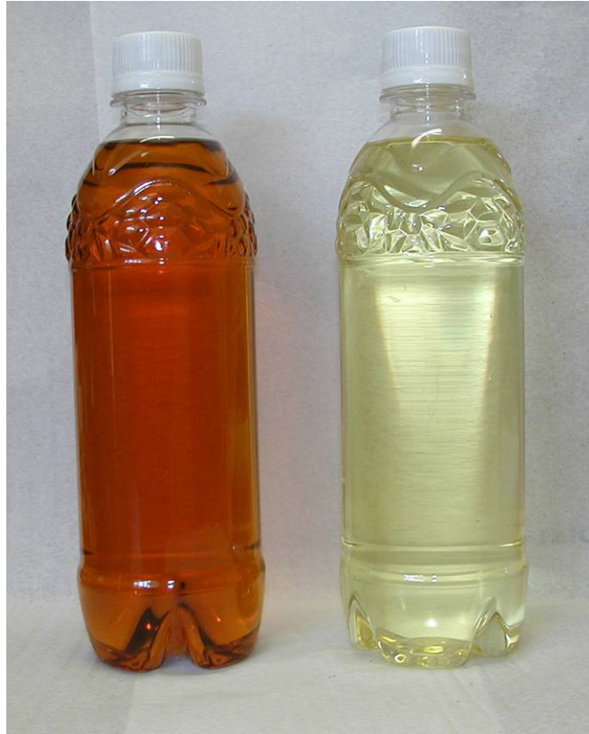
Figure 2-2: Biodiesel sample on left hand side and mineral diesel on the right
