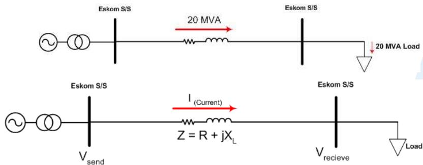
$$\text{Power}_{\text{loss}} = I^2 \times R$$
