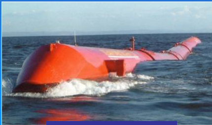
Pelamis 750 kW rating in 30m water depths
