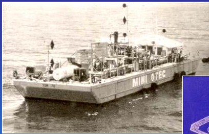
50 kW test platform off Hawaii (Mini OTEC)
