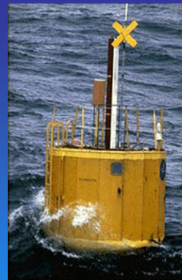
AquaBuoy 250 kW rating in 50 to 60 m water depths
