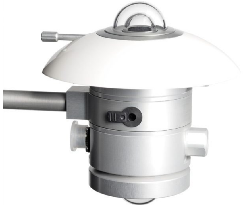
Albedo-meter – consisting of two standard pyranometers (preferred from a maintenance and calibration perspective)
