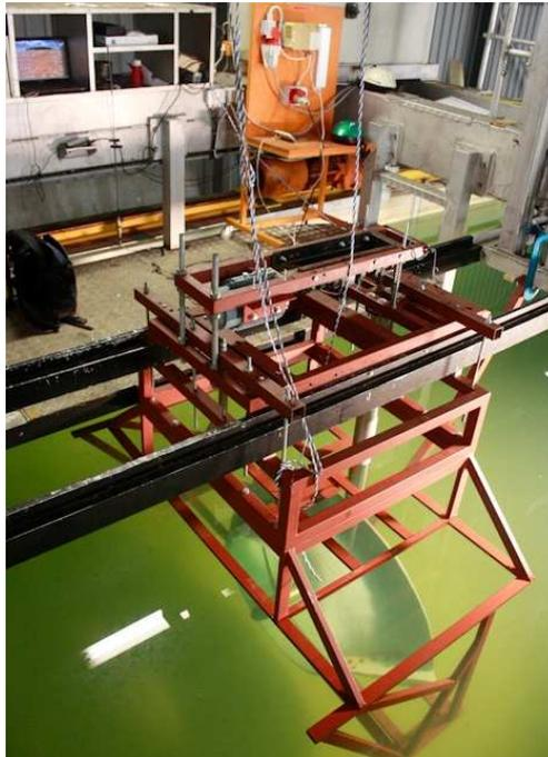
**Figure 5: Experimental setup in the towing tank facility**
