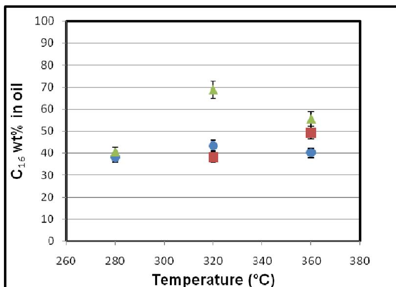
**Figure 4:** Effect of temperature on C<sub>16</sub> content in oil in a CO<sub>2</sub> atmosphere
