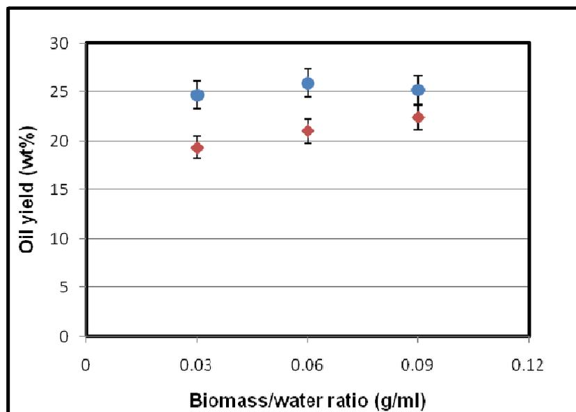
**Figure 3:** Effect of biomass/water ratio on oil yield
