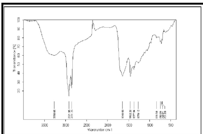
**Figure 5:** FT-IR spectra of bio-oil from liquefaction of *Scenedesmus acutus*.
