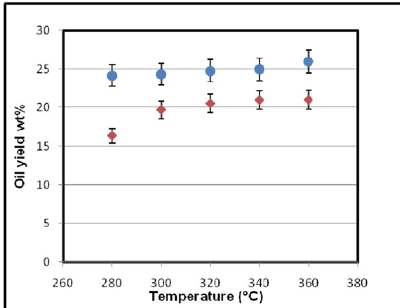
**Figure 2:** Effect of reaction temperature on oil yield.
