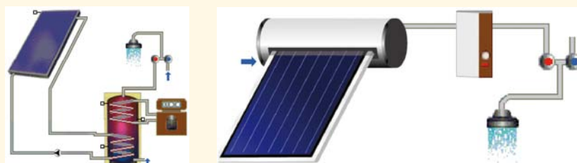
Figure 59, 60: Hydraulic scheme of the domestic hot water pumped reference system for single-family houses and hydraulic scheme of the domestic hot water thermosiphon reference system for single-family houses
