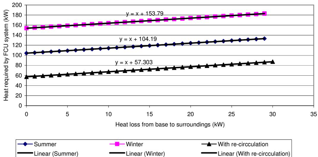
**Figure 9: Contribution required by the FCUs to meet heat losses from the base**
