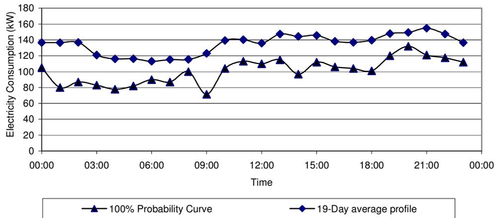
**Figure 5: Minimum electrical loads expected at SANAE IV**
