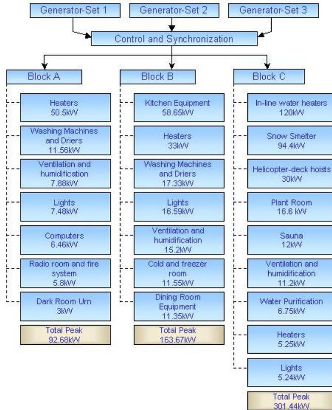
**Figure 4: Peak power demand breakdown of all electrical energy consumers**
