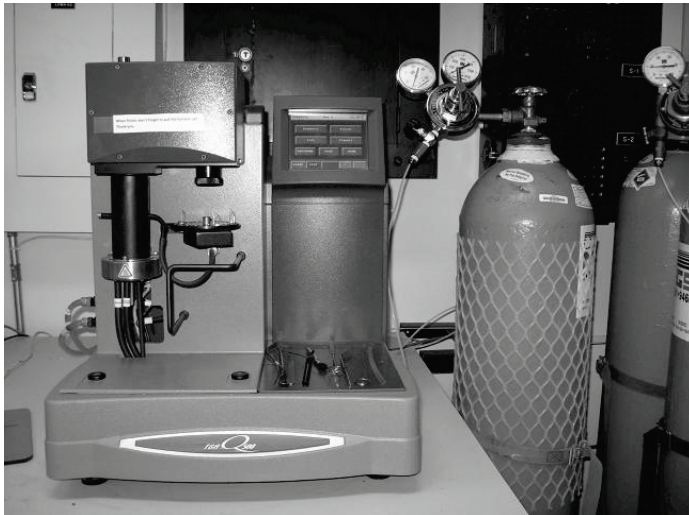
Figure 13: Q-500 Thermogravimetric analyzer
