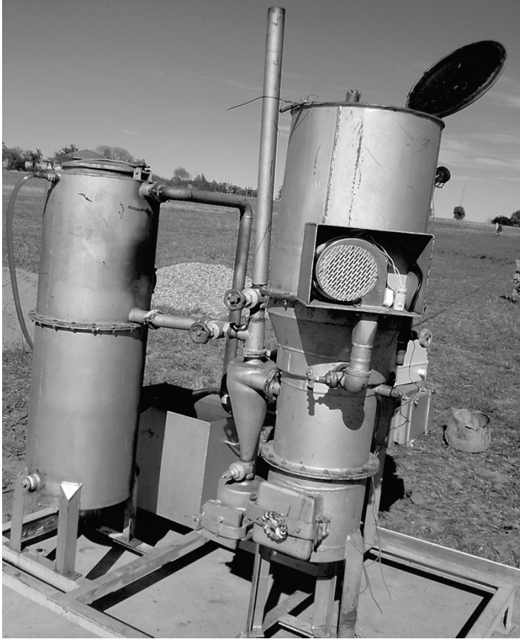
Figure 14: Prototype downdraft gasifier (open)
