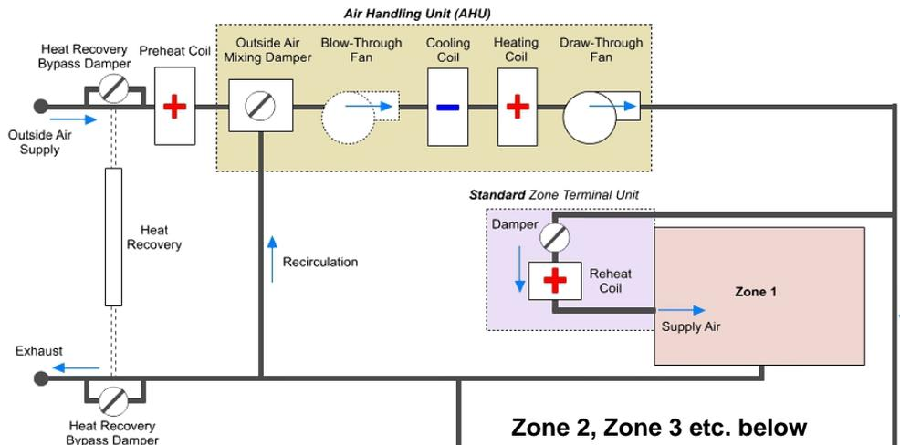
**Figure 21: VAV air handling unit (adapted from DesignBuilder, 2010).**
