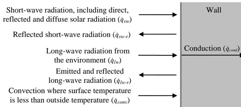
**Figure 11: External wall heat flux balance (adapted from EnergyPlus, 2010).**
