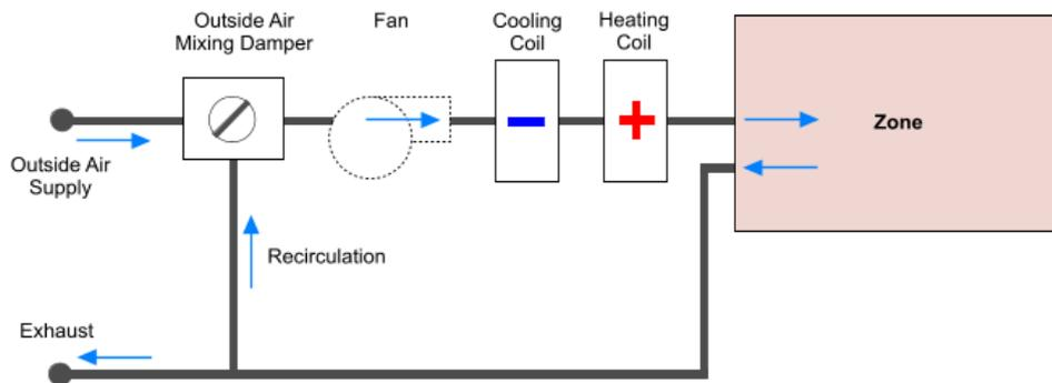
**Figure 19: Fan Coil unit (DesignBuilder, 2010).**
