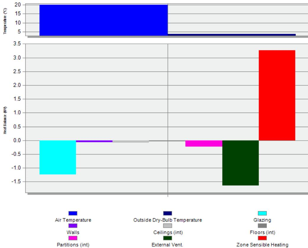
**Figure 43: Actual building Open Plan Office 2 winter design temperature and heat loss results.**
