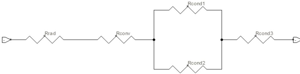
**Figure 13: Equivalent thermal resistance circuit of Figure 12.**
