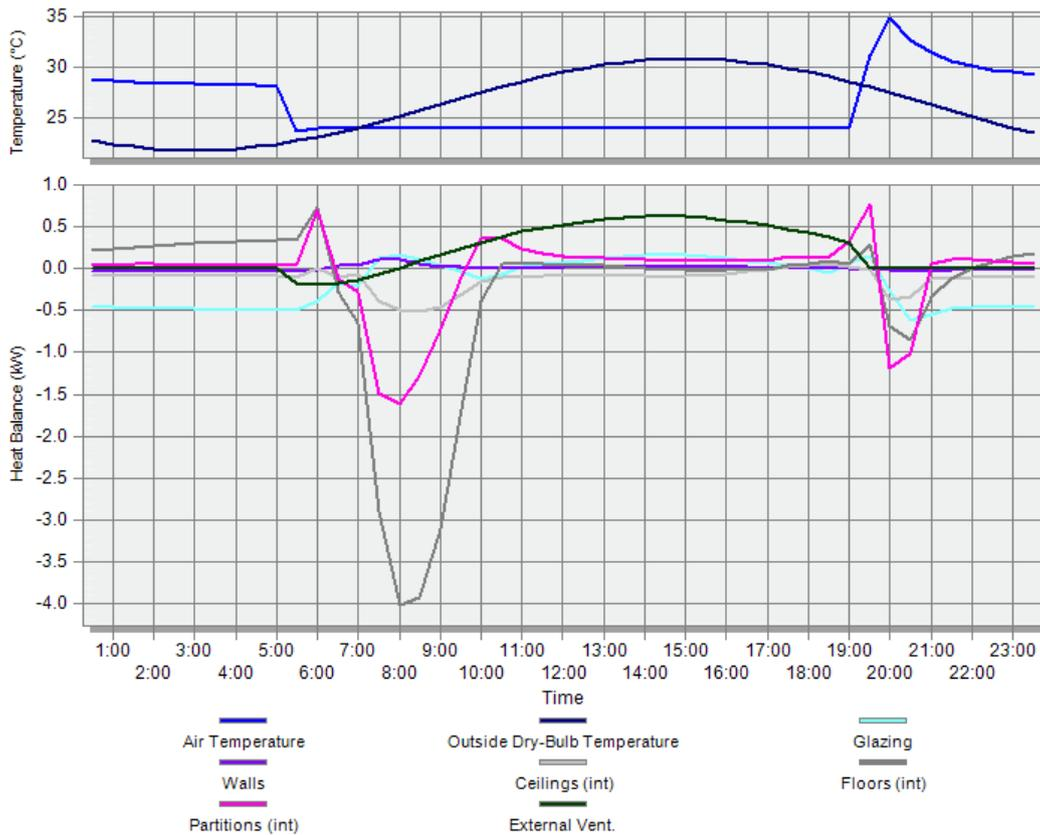
**Figure 42: Actual building Open Plan Office 2 summer design day fabric and ventilation performance results.**
