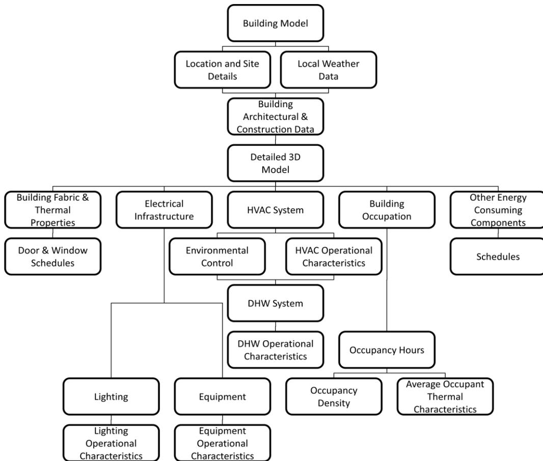
**Figure 14: High-level, quantitative physical building property-modelling breakdown.**
