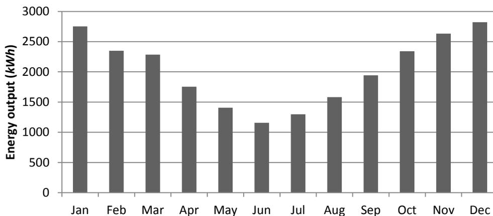
**Figure 45: PV array monthly energy output.**
