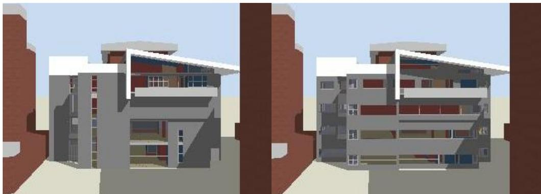
**Figure 20: 113° Façade glazing representation of the actual building (left) and the notional building (right).**
