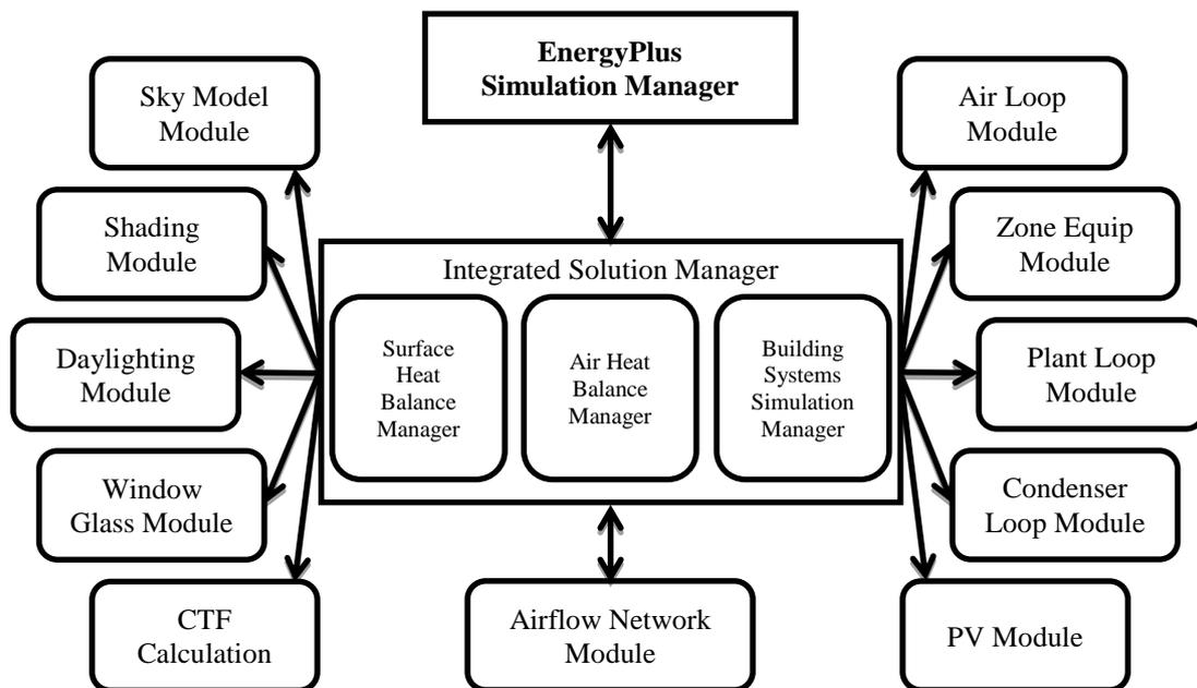
**Figure 8: EnergyPlus diagrammatical representation (adapted from EnergyPlus, 2010).**
