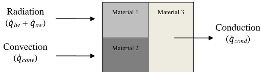
**Figure 12: Construction element material composition example.**
