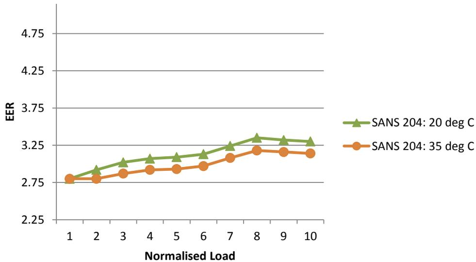
**Figure 22: Notional building chiller performance curve (GBCSA, 2011).**
