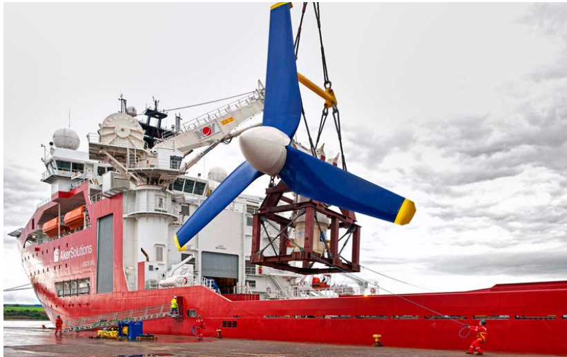
Figure 21: Atlantis Resources Limited turbine (Tethys, 2015)
