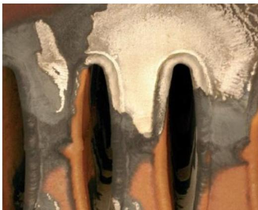
Figure 1.1: Corrosion on entrance to the ACC tubes
